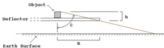
Figure 4-10 – Size Requirements for a Disk Shaped Deflector
